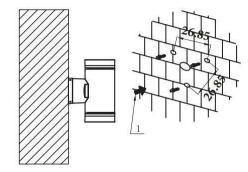
1)Drill 4 holes on the mounting surface according to the sizes shown on the above figure
