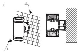
4)Fix the lamp onto mounting bracket5)Tighten the 4PCS screws to fix the lamp housing onto the installation surface
